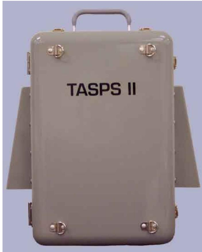
*TASPS is a portable system that uses navigational data acquired from multiple sources to switch radio antennas for maintaining solid satellite communication. The system utilizes dual GPS receivers and an electronic compass to ensure reliable functionality. TASPS is small enough to fit into limited spaces and light enough to be carried by a single person. The rugged design enables it to handle harsh ocean environmental conditions.*
