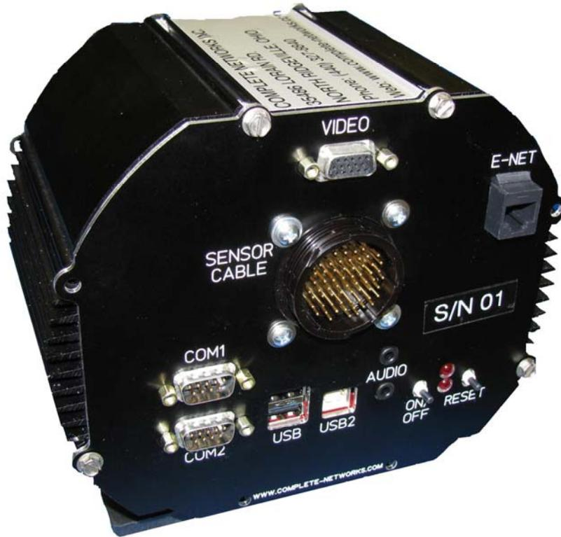
*The PC104 unit was designed and used for general purpose measurement and test. A typical application monitors sensors to facilitate control of motors and relays in a semi-automatic test environment. The Ethernet connection provides a mechanism for uploading test results to a centralized database.*
